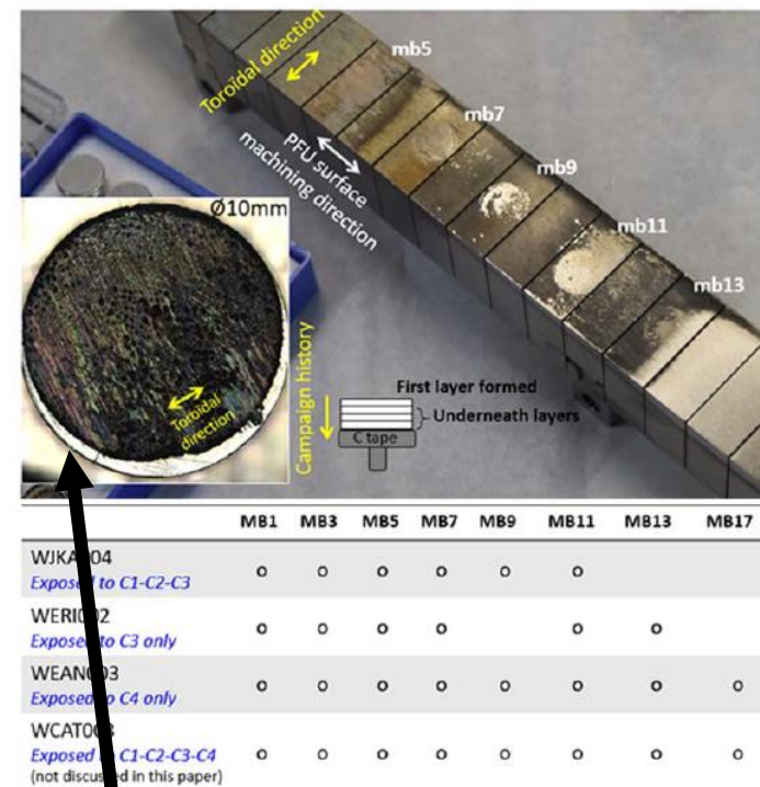
Figure 3. Photograph of PFU WEAN003 taken after the deposits have been collected using the SEM holder. Inset showing a photograph of the SEM sample holder with the deposit on the carbon tape. The table below details the MB's where deposits have been collected for each PFU.
